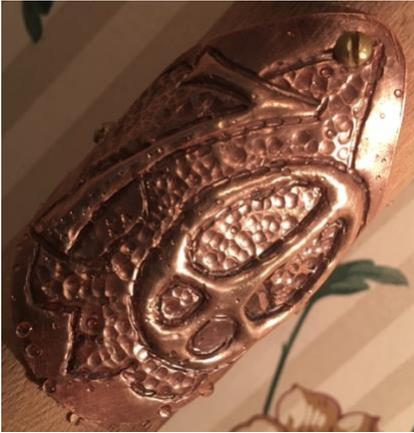
This course will introduce concepts, tools and methods of chasing and repoussé (or repoussage) (C&R). Consider a flat piece of metal: chasing yields a design on its side to be viewed, while repoussé pushes out material from the back to create visual depth in the finished piece. All working of a piece is done using steel punches and a hammer to move the metal to create a finished piece.
